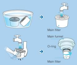
1. After 1 hour of soaking, take out the main filter from the water container, then flush water through the filter until no black or white small particles is present. (Tapping the filter from side to side may help to flush the filter more thoroughly). Then install the main funnel as shown. Please check if the rubber ring (O-ring) of main filter is properly installed. This may cause a leak.
