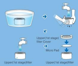
3. Soak for 1 hour, then remove the upper(1st stage)filter from the water container and flush water through the upper(1st stage) filter until no black or white small particles come out from the filter. Then place the micro pad on the upper(1st stage)filter, assemble the upper(1st stage)filter to the upper(1st stage)filter cover as shown. Please make sure that the micro pad is properly placed between the upper(1st stage)filter cover and the upper(1st stage)filter.
